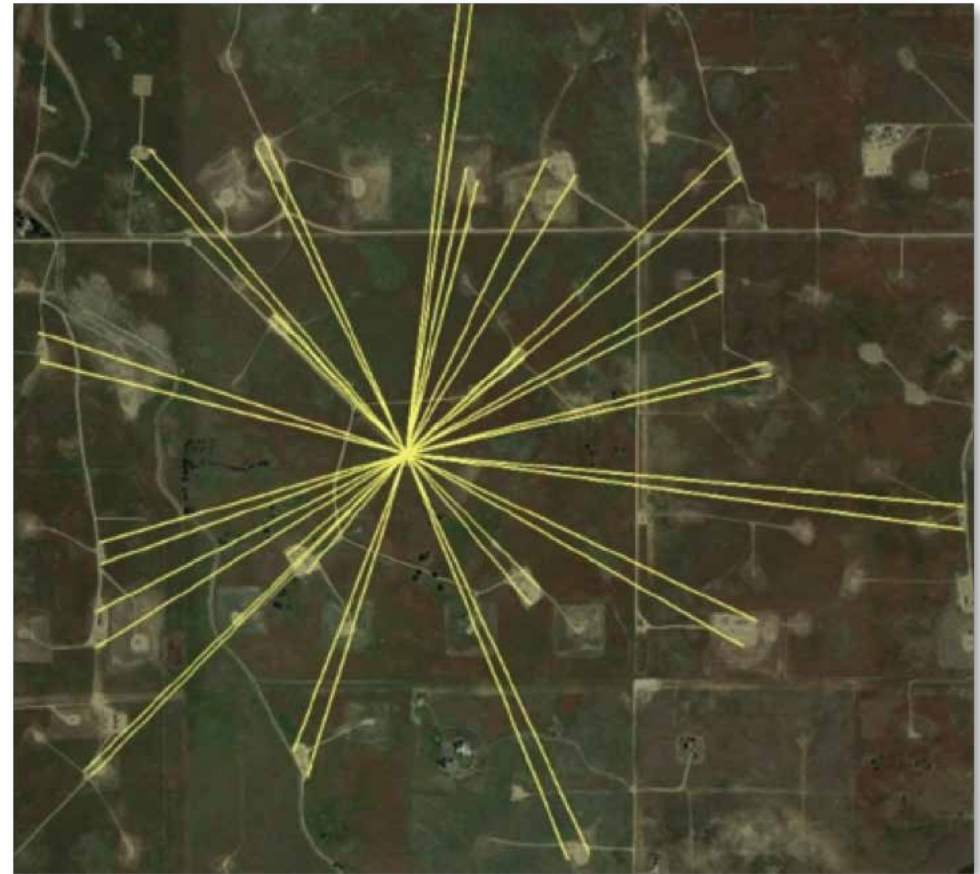
Centralized telescope monitoring node can detect emissions from multiple pads
